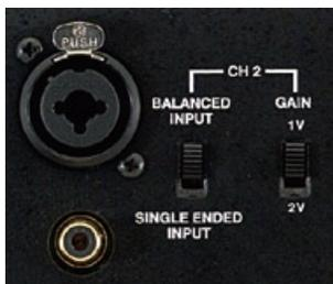
**Input flexibility: XLR or 1/4" phone jack for balanced signals and RCA jack for single-ended source; input gain is selectable.**
